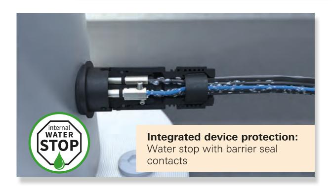
Experience shows Water gets inside the wiring system time and time again. The culprits are incorrectly executed installations, damage to wiring or temperature differences. Before long, the installation is penetrated from the inside by moisture damage. Installed barriers, which stop the water in its tracks, help here. The new **RST08i3** is optionally available with this function, each individual contact being sealed on the inside.
