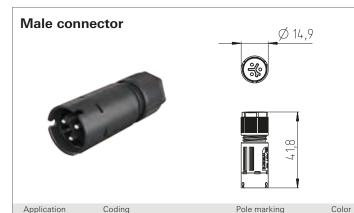
Unmounted with screwed cable gland. Suitable pin wrench for the cable connection, Accessories. For stripping lengths, refer to Technical Specifications. Cable assemblies on request
