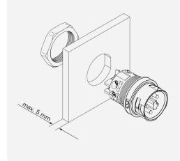
Dimension drawing of the opening for housing installation.
